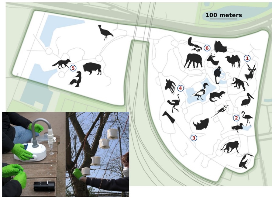
FIGURE 1 | Map of Rotterdam Zoo (the Netherlands) including the 6 sampling locations (numbered circles). Location 6 represents an indoor site. Photo inset depicts sampling setup of the Coriolis Micro (A), Pollensniffer (B), and the passive Nutshell eDNA samplers (subject is H. Jager) (C).
