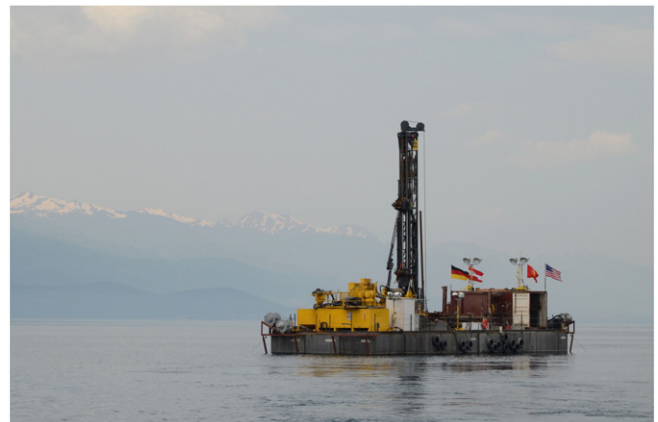
Fig. 2. Deep lake drilling system of DOSECC (USA) in operation at Lake Ohrid. In this case, the equipment had to be shipped from Salt Lake City (USA) to this inland lake on the Balkans.
