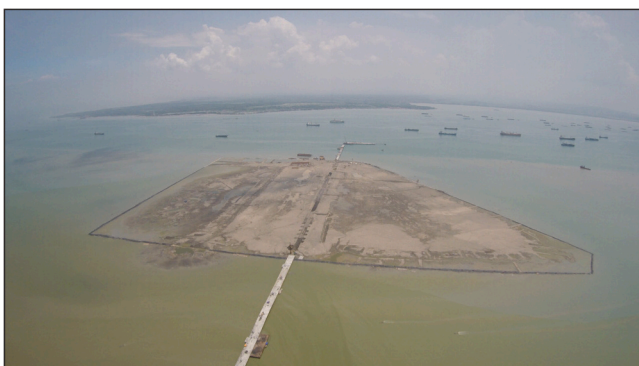
Fig. 2. The BMS island in the Madura Strait shortly after reclamation, June 2015. View to the east, toward Madura. Courtesy of Pelindo III.
