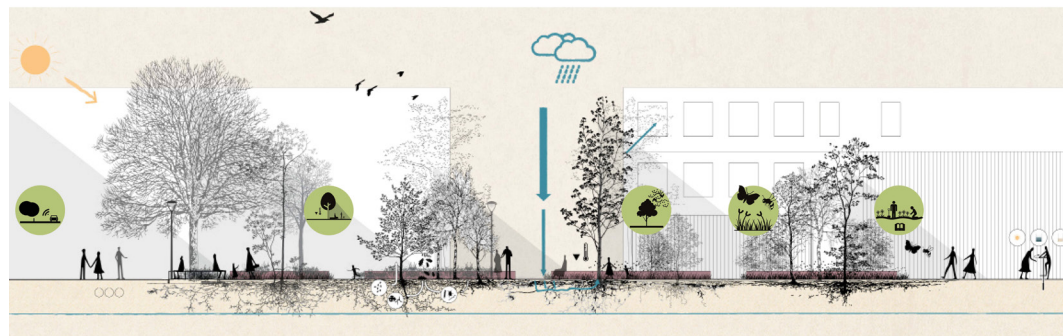
FIGURE 6 A design methodology based on observation. The degree of sunlight, shade, soil moisture characteristics, and soil type determine which natural habitat, its reference in South Holland, and its corresponding planting type are applicable for a specific urban location. Climate adaptation of the urban environment is therefore designed from the habitat of trees. Based on this initial analysis, three design principles were used in the pilots: A: soil demineralization, B: vital soil, and C: co-creation.
