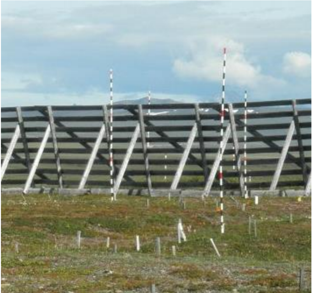
Figure 1.9. Snow fence - wooden fence ca 60 m long and ca. 2.8 m tall to accumulate snow brought by the predominant wind from Brooks range. Snow fences increase the snow depth from ca 0.5 m (ambient depth) to ca. 1 - 3 m depending on the distance from the fence.
