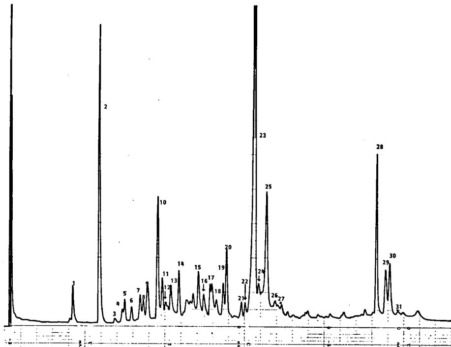
Fig. 2. Gaschromatogram of the crude extract of *Nipponolejeunea subalpina*. GLC condition: Column, SE-30 1% 3 m × 2 mm, column temp. 50–270° at 5°/min, inject. temp. 260°, He 30 ml/min.
