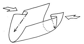
Fig. 14. Plunging minor folds resulting from stress oblique to the main structure.
