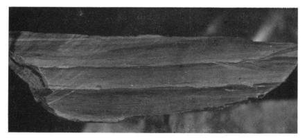
Fig. 10. Well-developed graded bedding in sandstone of Cervera Formation (x 1).
