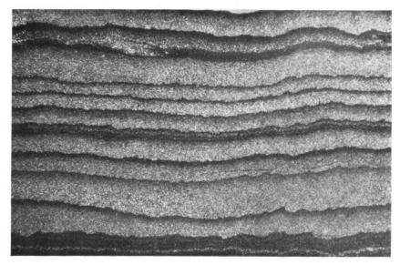
Fig. 7. Graded bedding in sandstones of Murcia Quarzite Formation  $(\times 10)$ .
