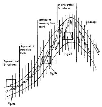
Fig. 26. The development of minor structures in different parts of a larger fold.
