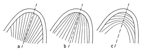
Fig. 20. Diagrams of cleavage relations in an anticline a) normal axial fan diverging upwards b) unusual axial fan converging upwards c) concentric cleavage.
