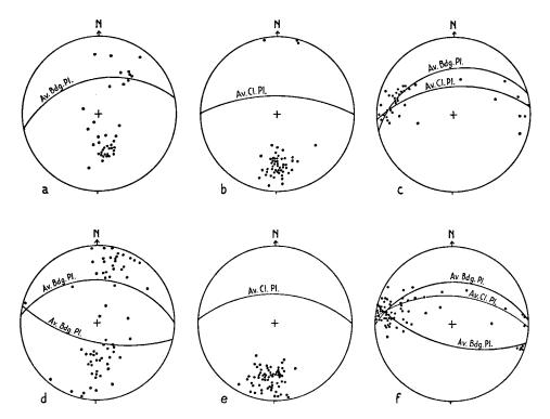
Fig. 17. Stereographic projections (Schmidt Net) of measurements from the Lechada Formation, Curavacas Syncline;
