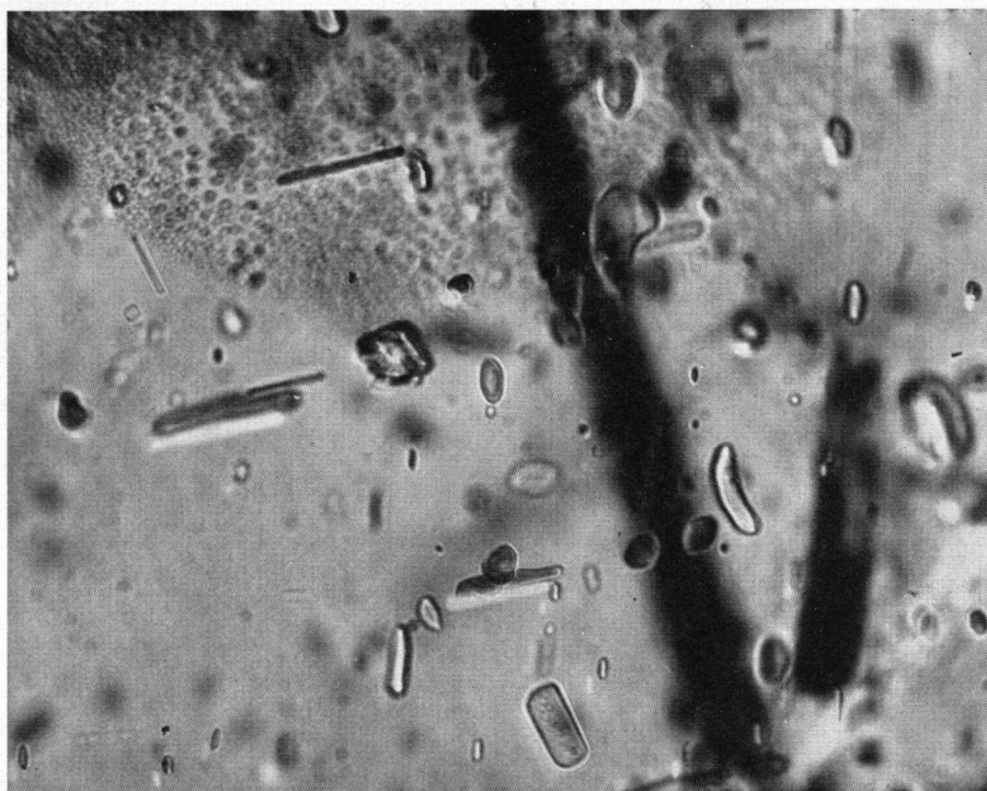
Fig. 5. Mica inclusions in peridot No. 722, at the top of the photograph part of a healed fissure may be seen ( \times 100 )
