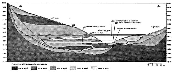
Fig. 10.5 Hydrogeological section along the Aiguamoix dam axis.
