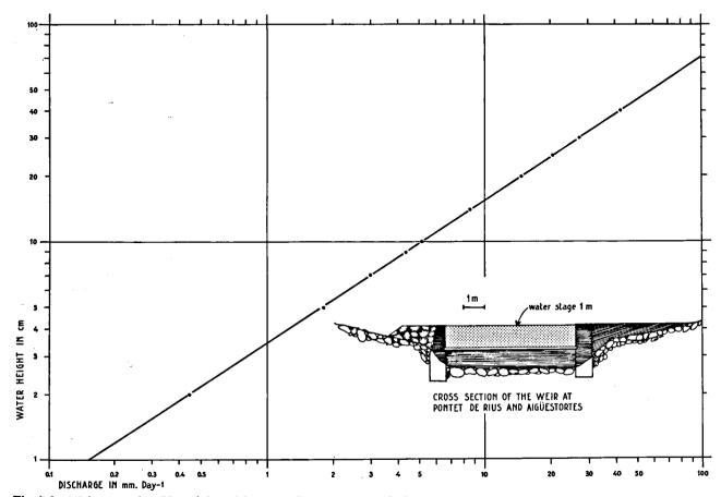
Fig. 7.5 Weir at station 20 and 3 and its stage-discharge rate relation.
