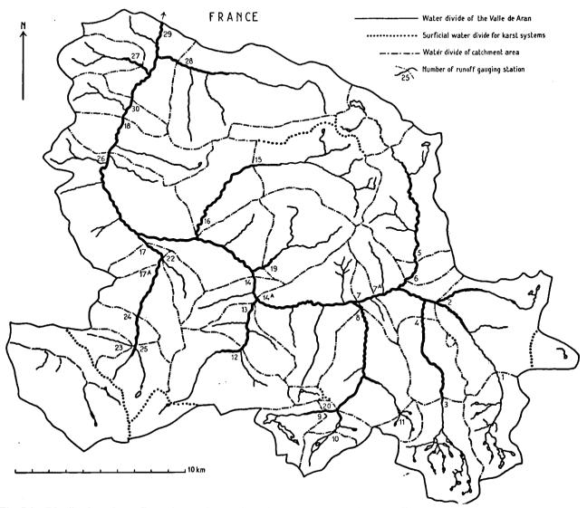
Fig. 7.1 Distribution of runoff gauging stations and catchment areas, showing the effect of karst systems.
