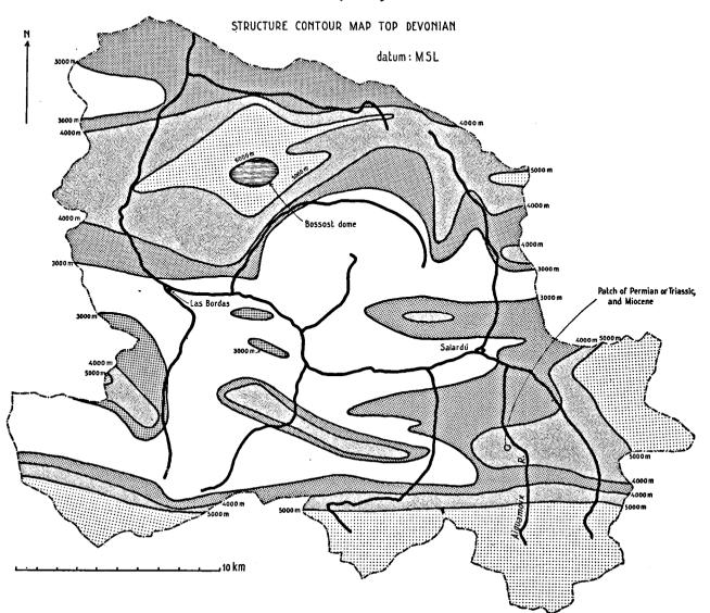
Fig. 2.8 Structure-contour map of the top Devonian in the Valle de Arán.
