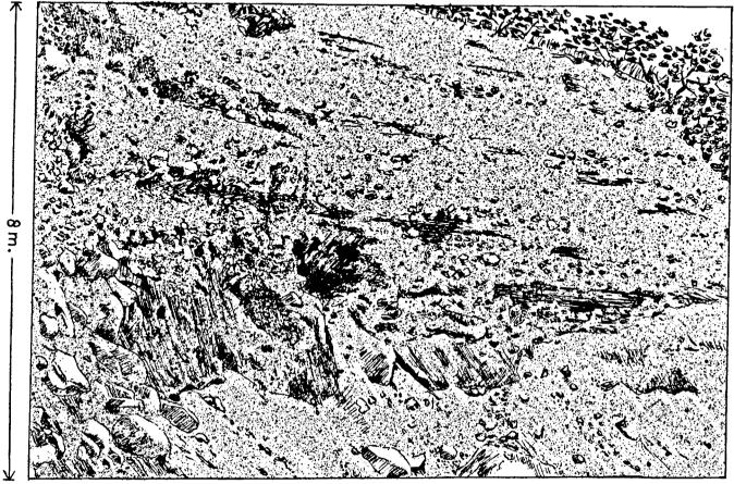
Fig. 10.3 Fluvio-glacial material in the left Aiguamoix bank, 700 m south from the dam
