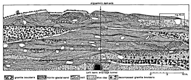
Fig. 10.4 Geological profile of the left Aiguamoix bank at the damsite.
