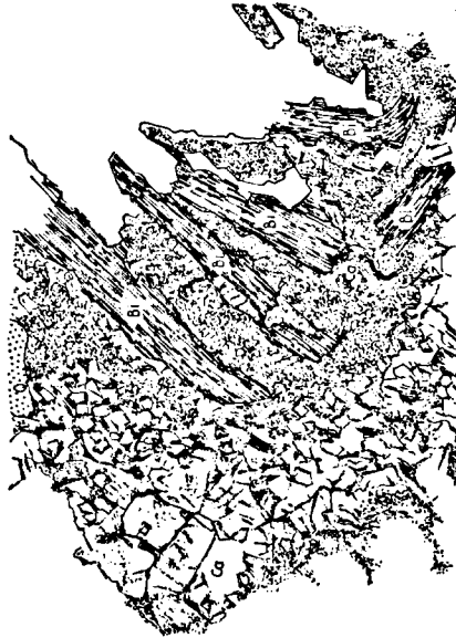
Fig. 4 Biotite grains, partly replaced by calcite (X 150, uncrossed nicols)
