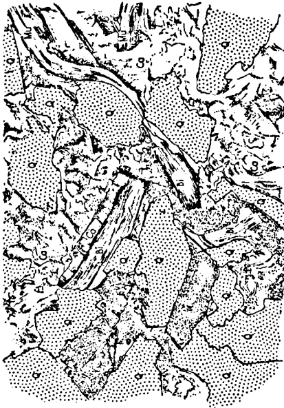
Fig. 1 Carbonate, lying against biotite in the centre of the picture, showing pseudomorphism after biotite (X 200, crossed nicols)
