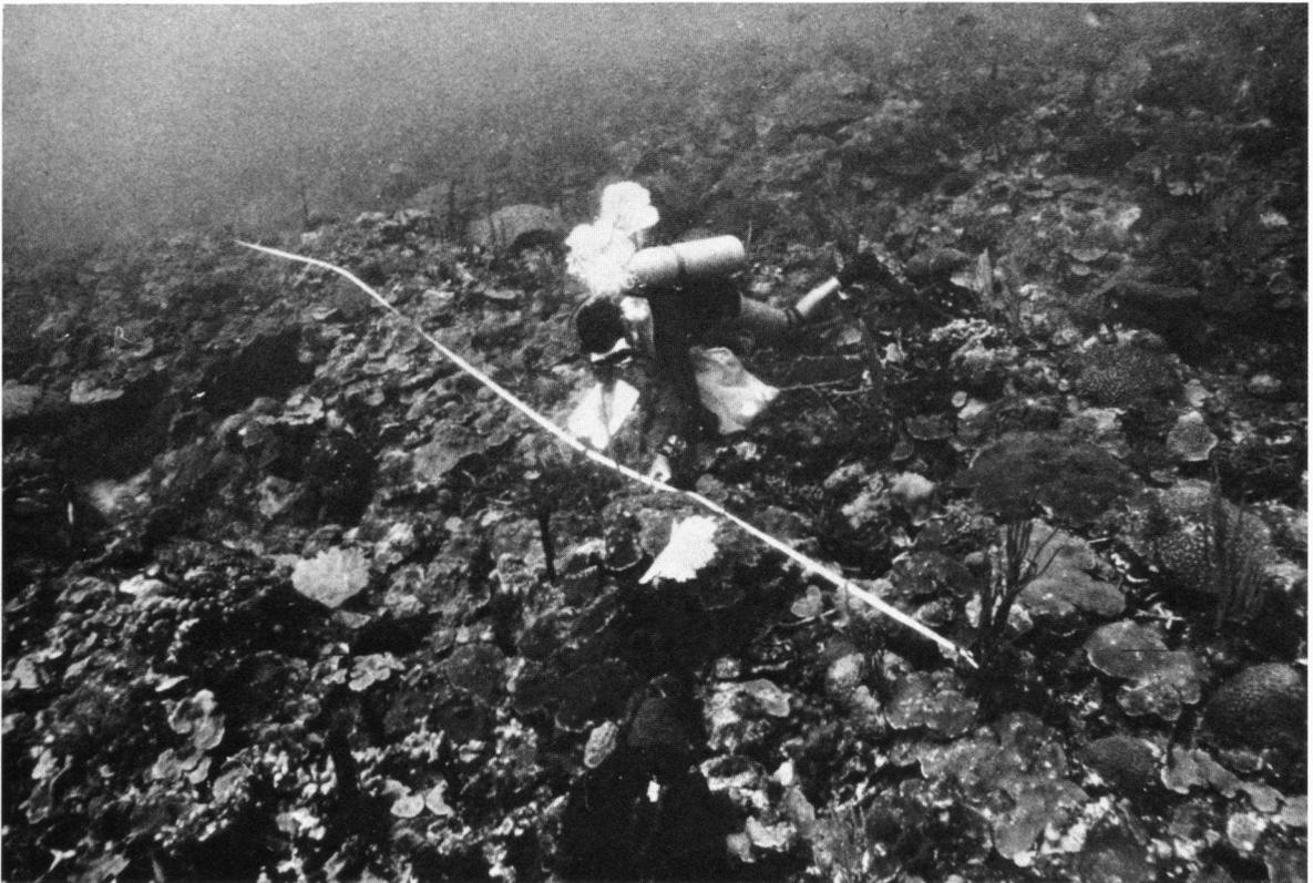
Fig. 7. Use of the measuring tape. LITR: the intercept-length of the line with each underlying bottom feature is noted. POLI: the bottom features underlying points at 20 cm intervals are noted.
