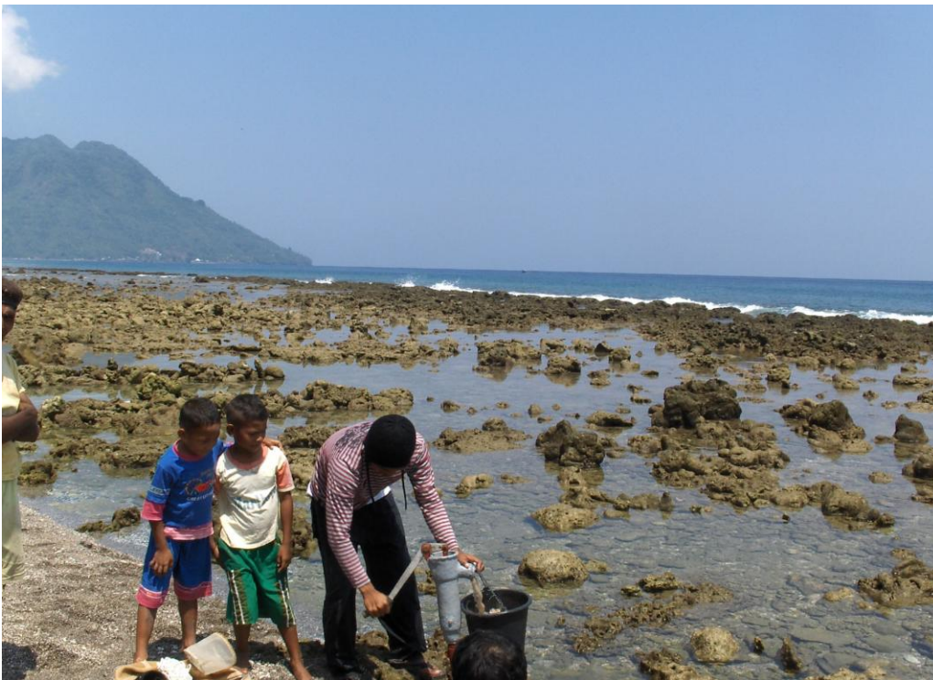
Photo: Bou-Rouch pump used on a marine beach. The suction creates an irregular inflow that detaches groundwater organisms from their substrate and brings them to the surface. Water is filtered through a net.
