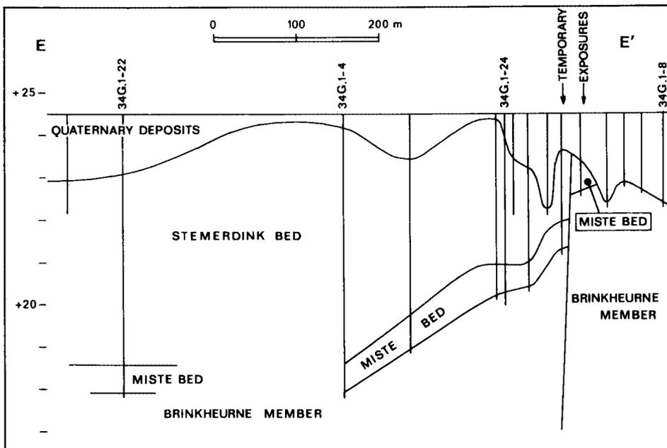
Fig. 11. Geological cross-section of the Aalten Member reference section (boring 34G.1-24). For a locality map see Fig. 10.
