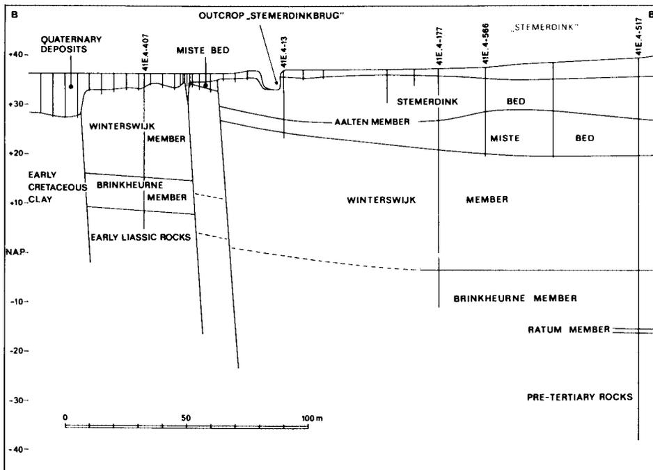
Fig. 9. Geological cross-section of the Stemerding Bed stratotype. For a locality map see Fig. 4.
