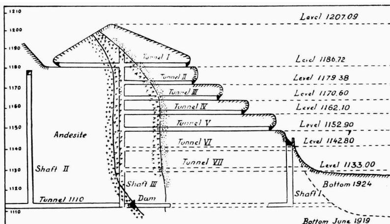
Fig. 7. The tunnels in the eastern crater wall of Mt Kelut (from van Hettinga Tromp, 1926; see also Stehn, 1929c, p. 19).
