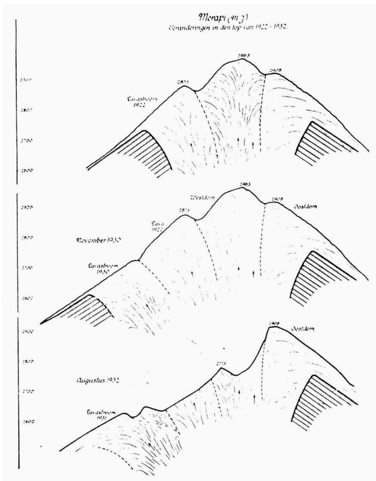
Fig. 9. Cross section through the summit of Mt Merapi, showing the dome of 1883 ('Oost-dome'), the West dome, the lava of 1922, the outflow of 1930, and the situation after the eruption of December 1930 (from Neumann van Padang, 1936b, fig. 5).
