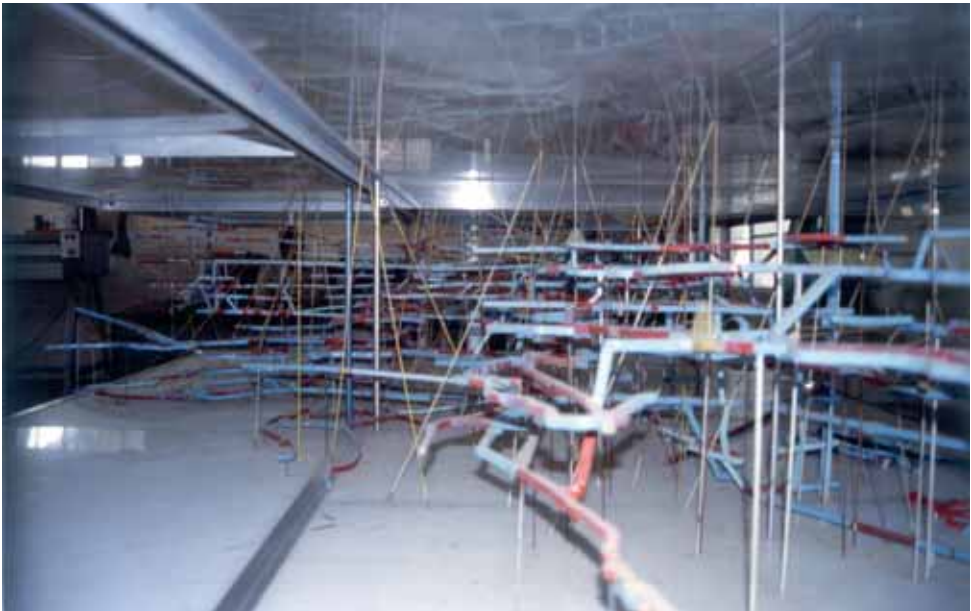
Fig. 26. Three-dimensional model of the underground mine workings at Zeus, showing all the tunnels and shafts that have been dug, and locations of pegmatites (marked in red) and emerald. The model is constantly revised.
