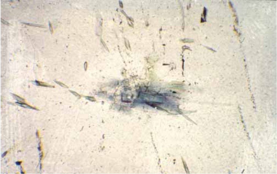
Fig. 52. Holmquistite frequently occurs in emeralds, which are formed in pegmatite. Length of this crystal is 300 \mu\text{m} .
