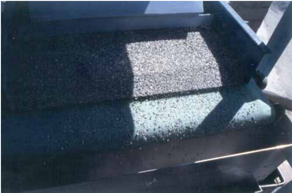
Fig. 31. The Permanent Magnetic Roller separates slightly magnetic schist from emerald and remaining schist. The emeralds fall off the conveyor belt, whereas the magnetic schist particles remain adhered to it.
