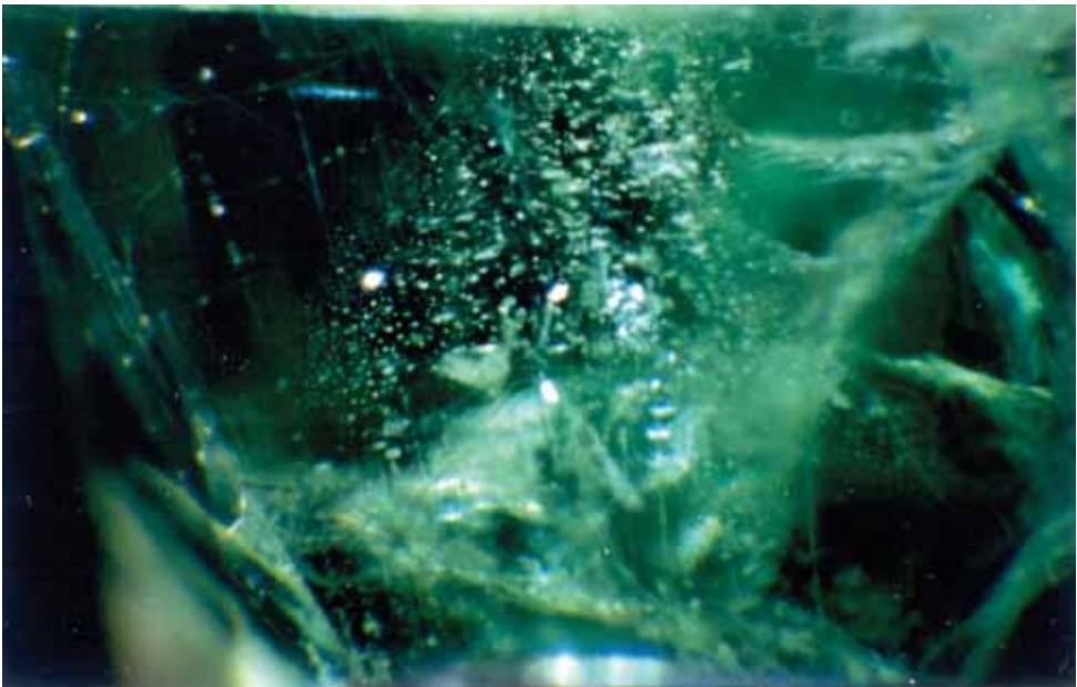
Fig. 56. Partially healed fractures containing minute inclusions were often present in the Sandawana emeralds examined. Darkfield illumination, \times 60 .
