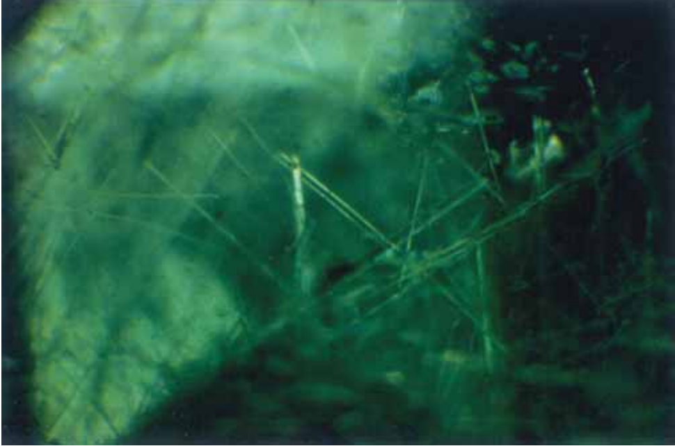
Fig. 40. The 'tremolite' needles and laths that are a well-known hallmark of emeralds from Sandawana were conclusively identified as actinolite and cummingtonite. Darkfield illumination, \times 50 .
