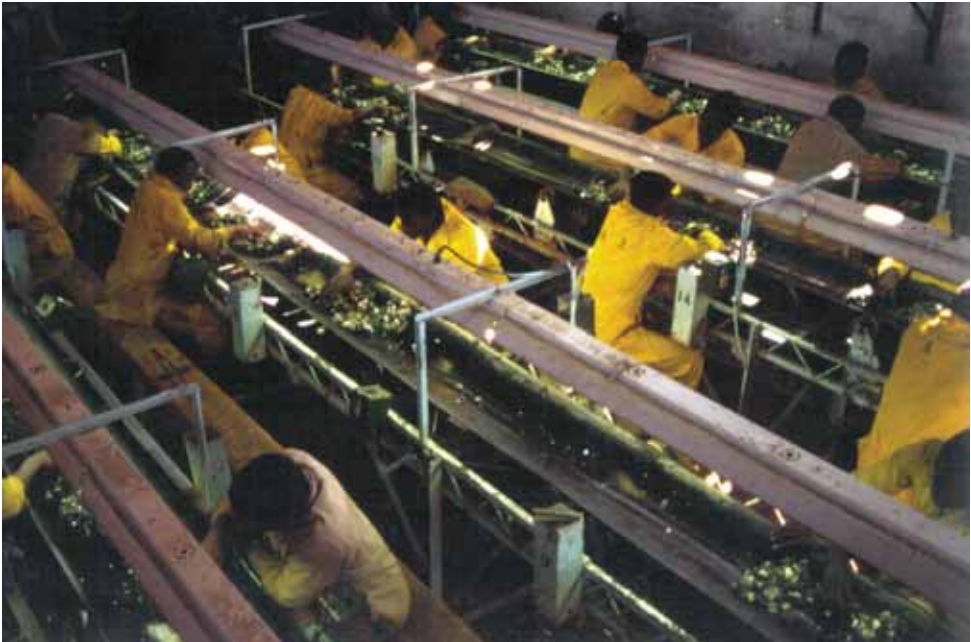
Fig. 29. Until a few years ago, all ore fractions on the slow-moving conveyor belts were carefully checked for emeralds by hand-pickers. Gem-quality pieces were deposited in safety boxes by each sorter.
