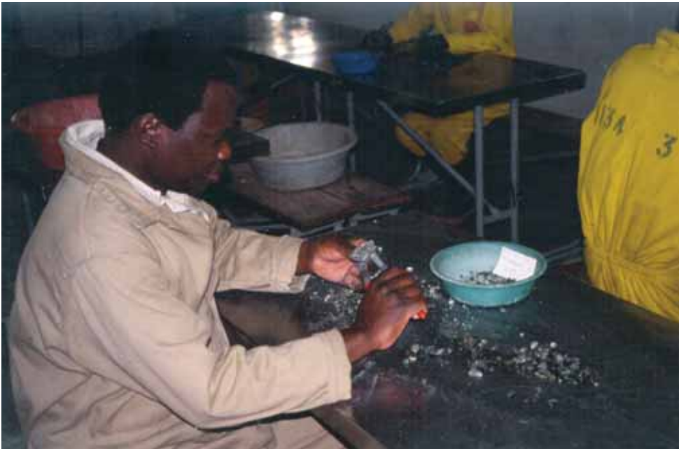
Fig. 33. Tungsten-tipped pliers are used to free the emeralds from their matrix.
