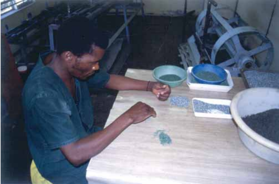
Fig. 32. In sorting rooms III and II the final ore is carefully checked by hand, and emeralds are sorted.
