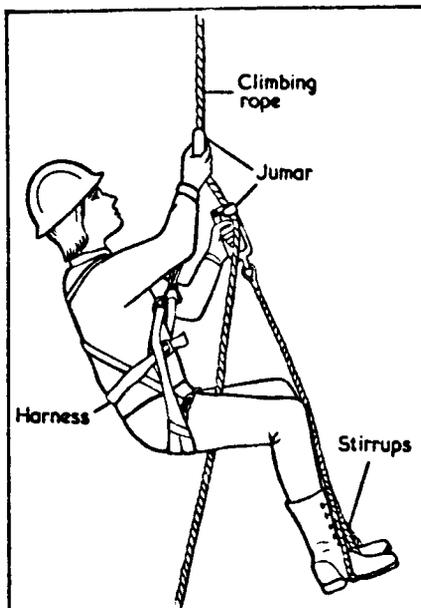
The climbing rope should be of a type used in caves, 8.5+ mm  $\emptyset$ , which is of the static type characterised by low elasticity. For climbing a pair of jumars (ascenders) are used, one of which is attached to a climbing harness, the other to a pair of footslings or stirrups (see figure). Climbing this way is not only easy, but also completely safe. For an easy descent a security 'stop' self-locking descender can be used.
