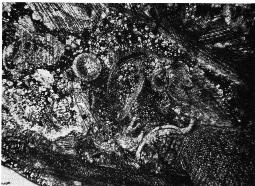
Fig. 28. Organo-clastic appearance of griotte limestone. Note presence of grain-growth calcite with syntaxial rims. 70 \times .
